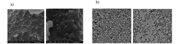
Fig. 1: Morphology of SMI nanoparticles: a) SEM b) TEM
