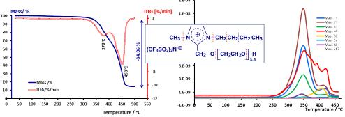
Fig. 1: Thermal stability of [BuMeIm 3.5EO]N(CF<sub>3</sub>SO<sub>2</sub>)<sub>2</sub> imidazolium ionic liquid.
