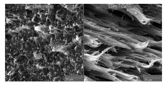
Fig. 1: The effects of nanofillers SiO<sub>2</sub> and CaCO<sub>3</sub> (5 wt%) in pure LDPE matrix
