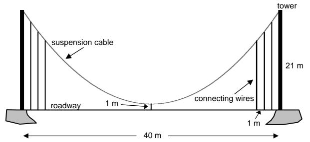
It is essential that the lengths of the connecting wires should be *exact*, otherwise the bridge is unsafe! The lengths cannot be found by *practical measurement while* building the bridge! This is how engineers do it: They imagine a system of axes, find a *formula* for the shape of the suspension cable, then they use this formula as a *model* to *calculate* the lengths of all the connecting wires *beforehand*.
