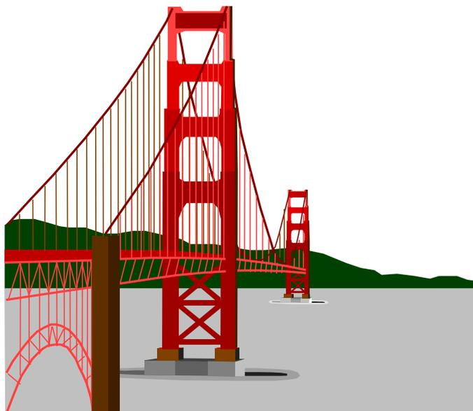
Engineers must build a hanging bridge over a river. The roadway of the bridge will be hung from a suspension cable with connecting wires, 1 m apart. At its lowest point, the connecting wire is 1 m long. The suspension cable is supported by two towers at the ends, which are each 21 m high and are 40 m apart.
