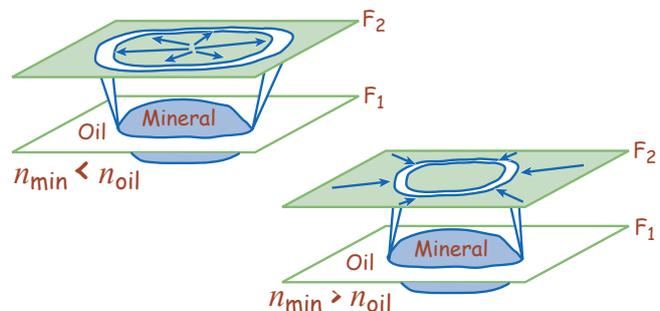
If  $n_{min} < n_{oil}$ , the cone diverges upwards and if  $n_{min} > n_{oil}$  the cone converges upwards. If the stage is lowered, the plane of focus goes from  $F_1$  to  $F_2$  and the Becke Line appears to move towards the material of the higher refractive index.
