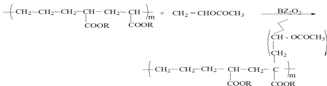
Figure 1: Scheme of Grafting of Vinyl Acetate (VA) on Poly Ethylene Acrylic Acid (PEAA) Co-polymers
