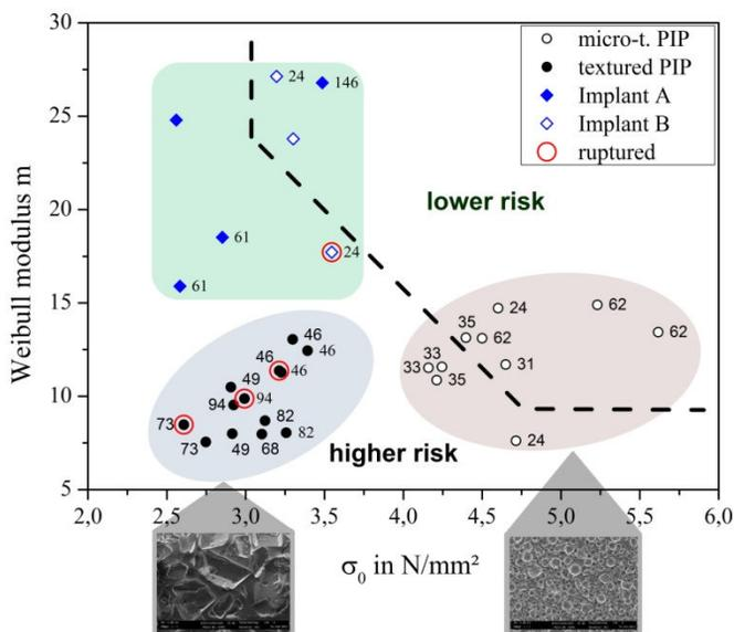
**Fig. 1:** Novel map, utilizing determined Weibull modulus  $m$  and characteristic strength  $\sigma_0$  as appropriate coordinates to benchmark implants manufactured by PIP, Benchmark A and B. The dashed line indicates a first guess separating good and poor quality implants. Numbers on dots are the duration of implantation, respectively.
