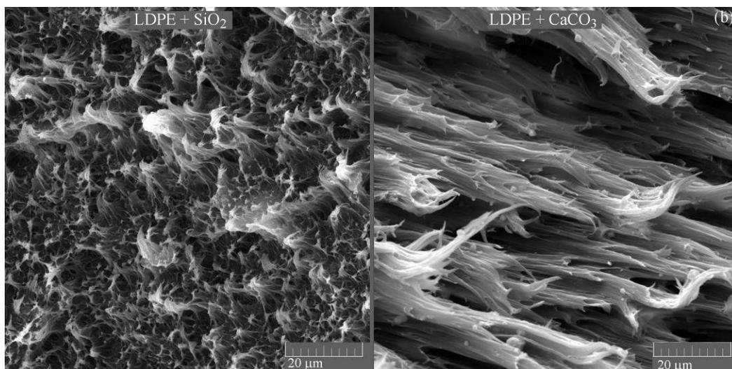
**Fig. 1:** The effects of nanofillers  $\text{SiO}_2$  and  $\text{CaCO}_3$  (5 wt%) in pure LDPE matrix
