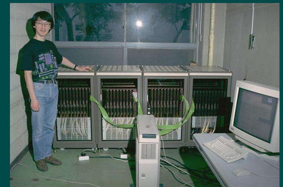
GRAPE (GRAvity PipE) special-purpose force-summation computer J. Makino et al. – University of Tokyo
