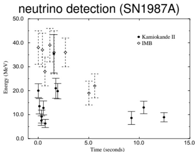
The Kamioka and IMB detectors are water Cerenkov detectors. Observed have been  $\bar{\nu}_e$  neutrinos via their interaction on protons (in the water molecule). The detection of the other neutrino types is the main goal for the next nearby supernova to test the predicted neutrino hierarchy.
