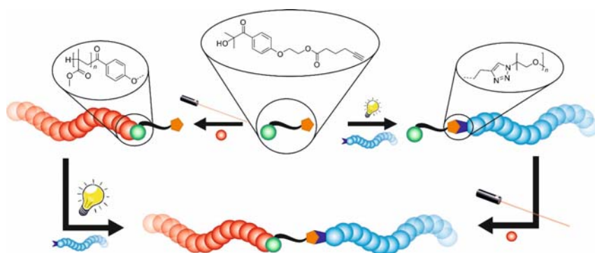
Fig. 1: A bifunctional photoinitiator is presented that can undergo CuAAC and free radical polymerization \lambda -orthogonally.
