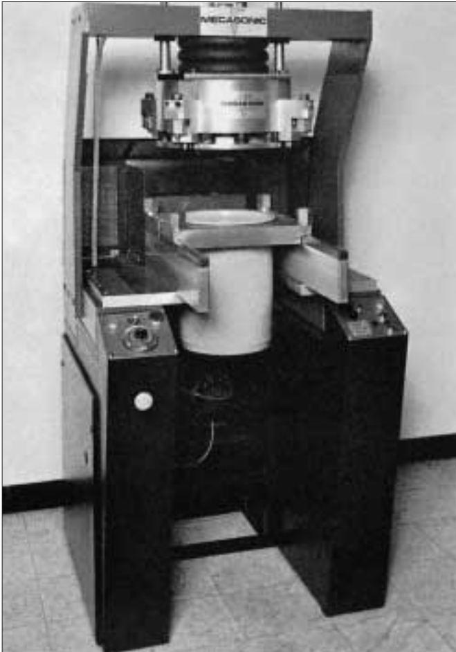
Fig. 10.90b Commercial linear and angular welding machine. Manufacturer: Mecasonic SA, Zone industrielle, Rue de Foran, Ville-la-Grand, Case postale 218, 74104 Annemasse Cédex, France.
